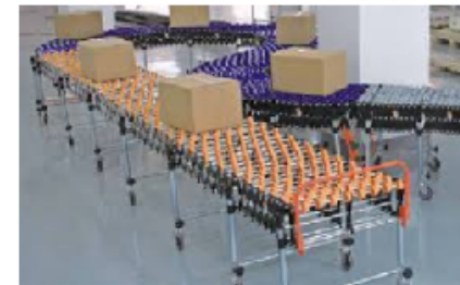
Roller Conveyors are ideally suited for moving products in a manufacturing line or warehouse, that otherwise may not be handled on a Belt Conveyor.
